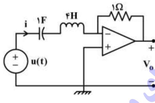
$$\frac{d^{\gamma}V_o}{dt^{\gamma}} + \frac{V_o}{\gamma} = -u(t) \quad (1)$$
