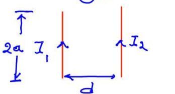
$$\vec{F}_2 = \vec{J}_2 \vec{l} \times \vec{B}_1 , \quad \vec{B}_1 = \frac{\mu_0 I_1}{2\pi d} (\hat{x})$$
